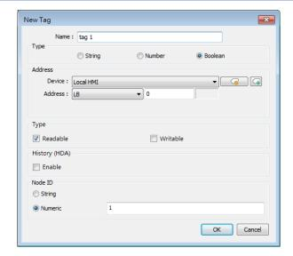
Add a new tag for the client to monitor or control. Two types of tags can be added: Data Variable and Property.
