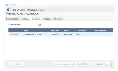
Note: According to OPC UA specification, an OPC UA client, in making a connection, will use a client certificate which will be checked by the OPC UA server for its legitimacy. The exception is if the security policy allows for the "None" option.
